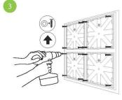
Make sure the arrows are pointing upward when mounting baseboards. Use a screwdriver or power tool to screw in. There are 16 screw points on each baseboard. They are located on the corners of each inner-square bracket.
