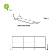
Be sure to start from top to bottom, When removing front panels
