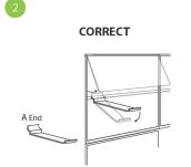
To remove the upper front panels, insert A end of the removal tool to the lower portion of the front plate. Use the lower front panel as leverage, then pull downwards.
