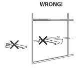
**WARNING:** Do not have removal upside-down when removing front panels. Improper usage will result in damage.
