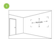
Using a measuring tape, measure the length and width of your wall to determine your desired number of baseboards.
