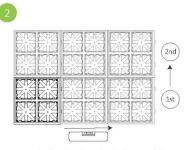
Mount the first baseboard at the bottom left corner, and work your way rightward. After you finish the 1st row, proceed to the 2nd row upward.
