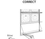
To remove the bottom front panels, insert B end of the removal tool to the lower portion of the front plate and push inwards.
